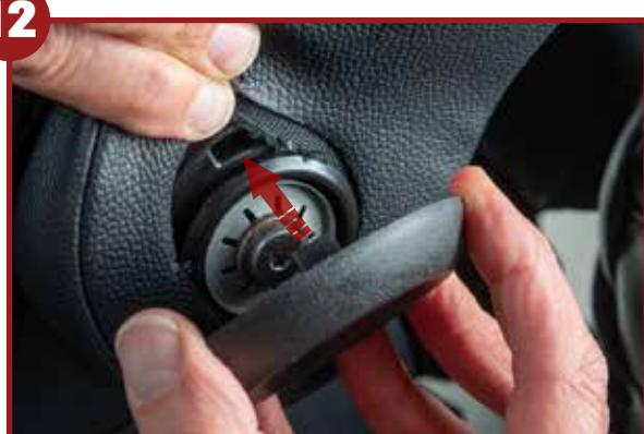
Tuck the material underneath the hinge cap, and reattach cap
