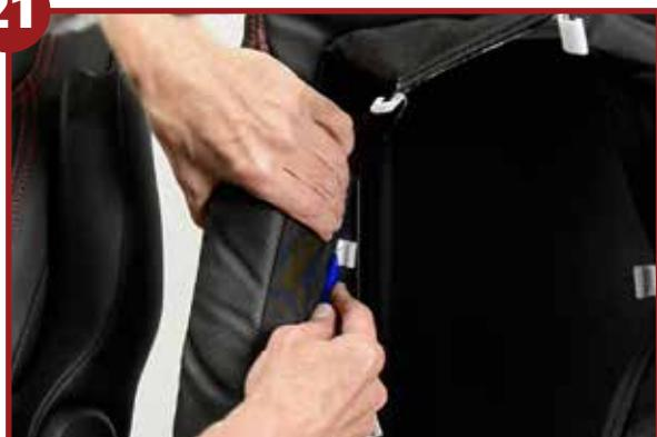
Attach the plastic hook behind the pull down tray panel
