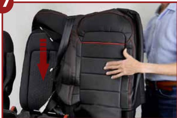
Slide the back covers over the back of the passenger seats
