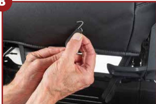
Attach hooks to the elastic bands on the bottom of the cover
