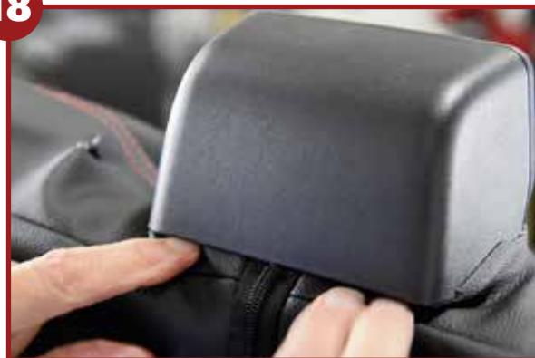
Tuck the material underneath the seatbelt housing
