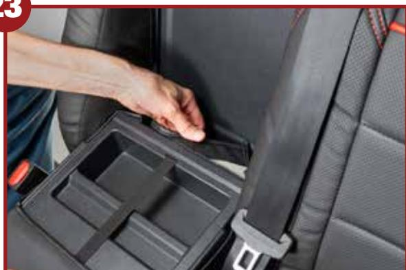
Pull through velcro and attach securely at the base of the tray
