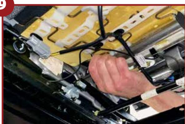
Attach the hooks to the underside of the seat securely
