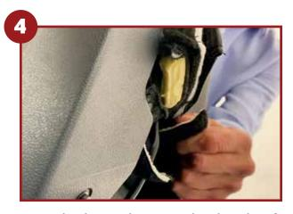
Attach the velcro at the back of the driver's seat
