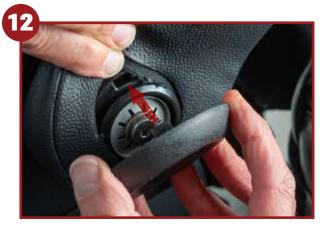
Tuck the material underneath the hinge cap, and reattach cap
