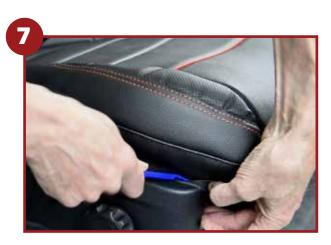
Tuck the material into sides of the seat moulding
