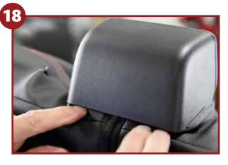
Tuck the material underneath the seatbelt housing
