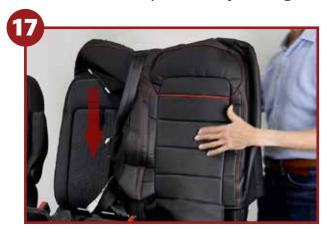
Slide the back covers over the back of the passenger seats
