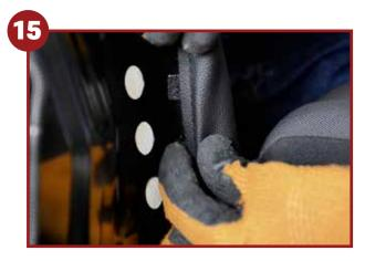
On the underside, fold the tab underneath upholstery fixing
