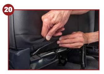
Attach the velcro securely at the back of the seats
