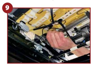
Attach the hooks to the underside of the seat securely
