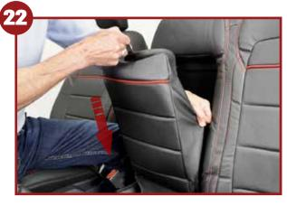
Slide the tray cover on, pulling through the fabric loop
