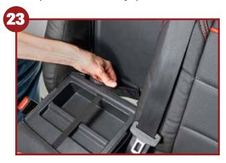
Pull through velcro and attach securely at the base of the tray
