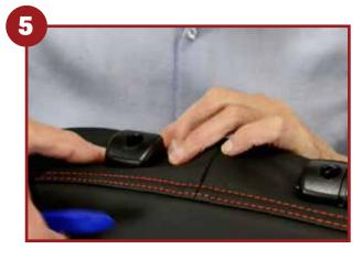
Push the material underneath the headrest guide inserts
