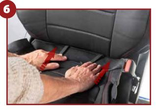
Push the driver's seat base cover through the seat join
