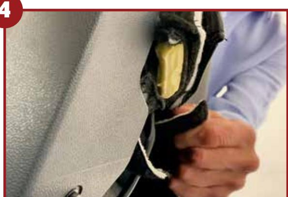
Attach the velcro at the back of the driver's seat
