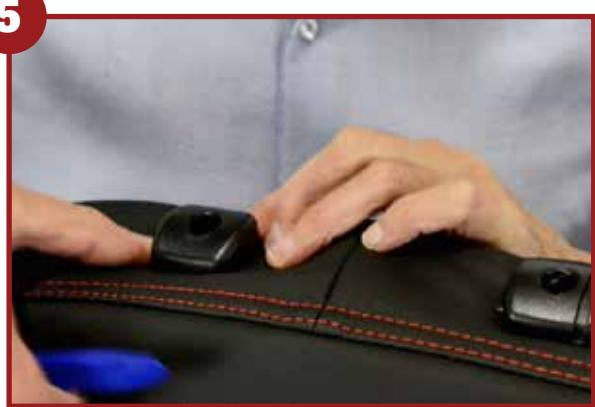
Push the material underneath the headrest guide inserts
