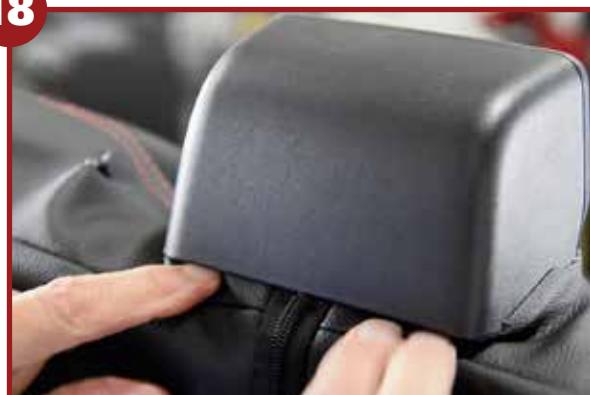
Tuck the material underneath the seatbelt housing
