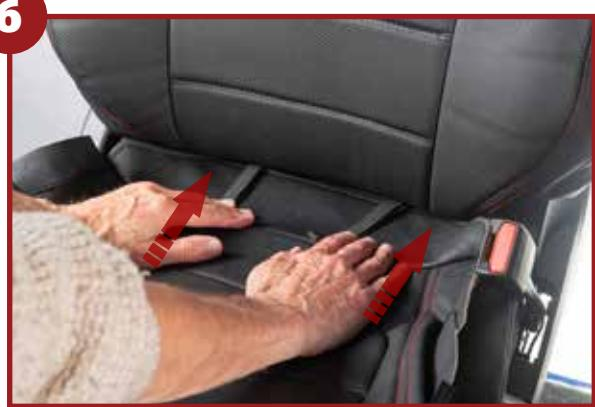
Push the driver's seat base cover through the seat join
