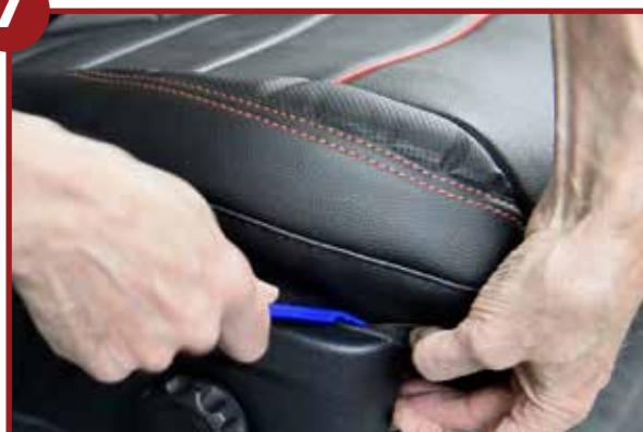
Tuck the material into sides of the seat moulding
